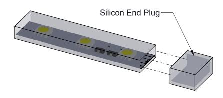
**STEP 3:** Trim the aluminum extrusion to be 7/16" shorter than the end of the pathfinder light.
