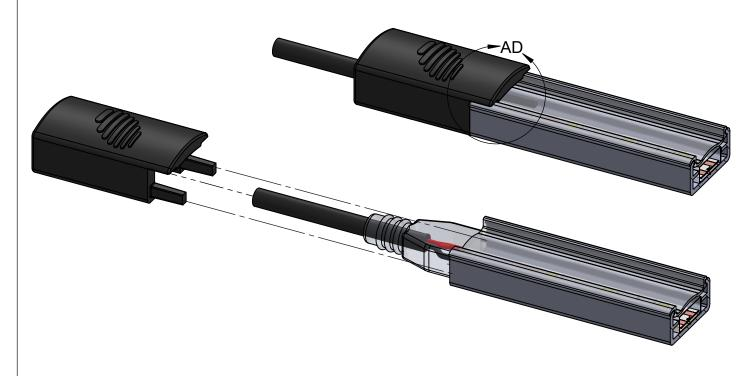
**STEP 9:**Slide the opposite end cap from the end and gently tap with a rubber mallet until the endcap is flush with the aluminum bracket.
