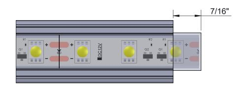
**NOTE**: More than one aluminum bracket and lens extrusion will be required for orders where the desired length is greather than 100".
