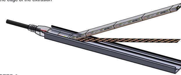
STEP 6: Unroll the pathfinder light into the aluminum bracket, pulling the adhesive backing as you go
