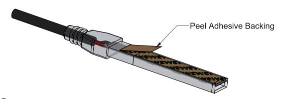
**STEP 5:** Place the pathfinder ribbon into the aluminum bracket, with the silicon endcap flush against the edge of the extrusion
